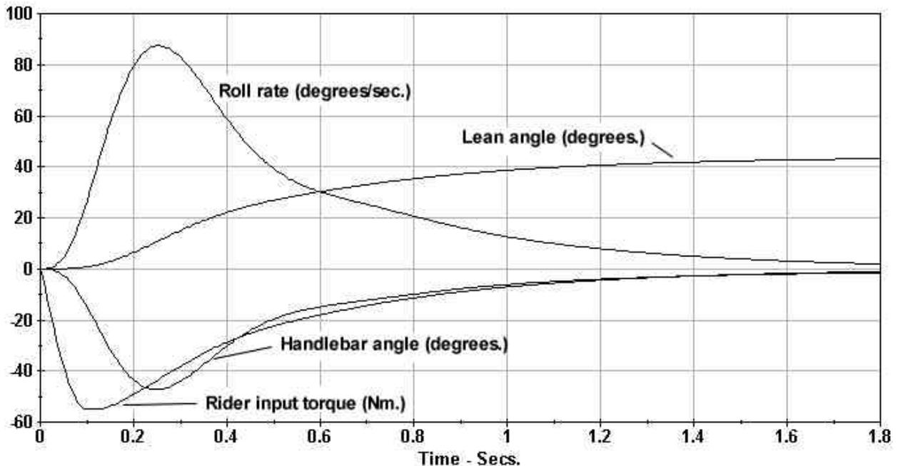
Fig. 4.6 Lean-in performance with no lateral tyre forces. Note how the leaning velocity or roll rate builds up to a
