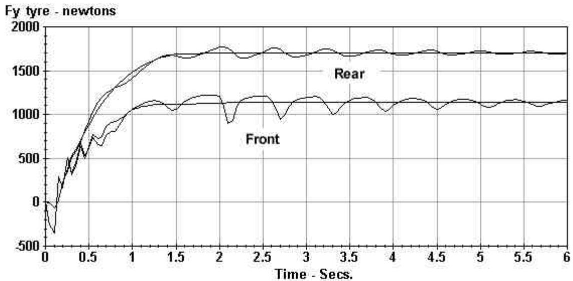
**Fig. 6.??** Lateral tyre forces. Even though it is the rear that is under-damped there is more variation on the front.
