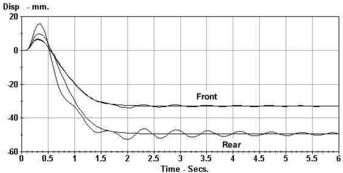
**Fig. 6.??** Front and rear suspension movement, showing the variation in the under-damped case. Note also the suspension extension during the first 0.5 second, this is due to the centrifugal force from the initial build up of roll velocity before the cornering force has overcome it and caused the compression. The damping value also affects the amount of this extension.
