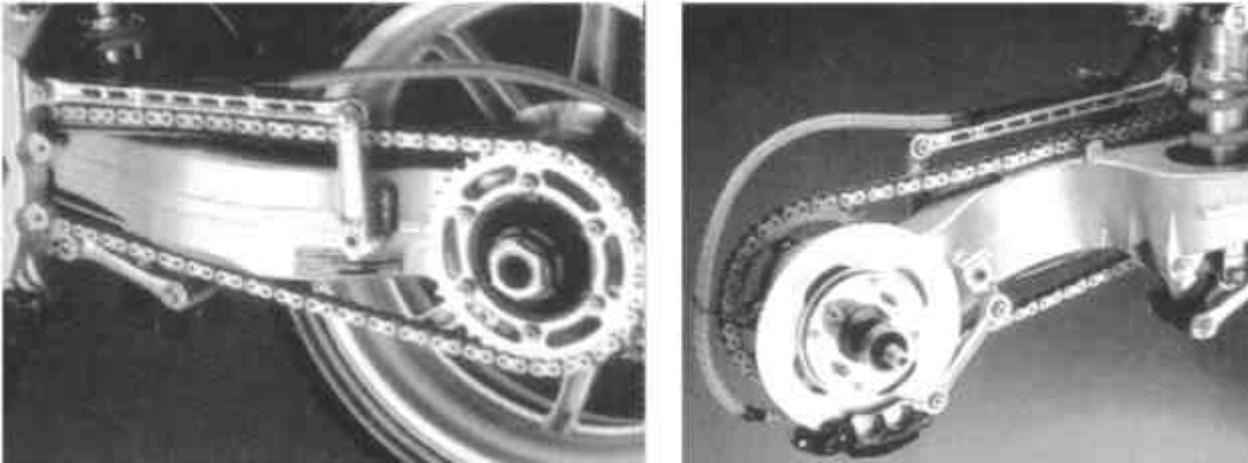
Chain drive single sided arm, interpretation by Honda. Note the levers each side of the arm just in front of the sprocket and brake disk, these take the torque from a floating brake caliper back to the main frame. Just like a normal floating caliper this gives control over the degree of squat. In order to mount the wheel bearings between the sprocket and disk the arm is quite complex in shape. This design necessitates a rotating axle which is large in diameter and hollow.
