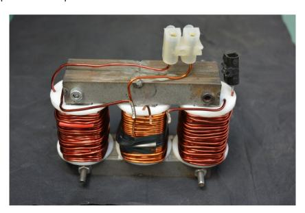
Once proven to have some beneficial effect, the filter needed some finishing off to make it suitable for everyday use. The coils were wrapped in strips of cotton material sourced from her indoors and dunked in varnish for an hour each.
