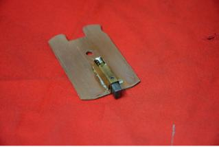
There were four machined and tapped holes in a great place to bolt the brush assembly. I shaped the printed circuit board so that it would fit against a cast in boss to prevent rotation with a single mounting bolt.
