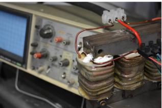
Studying the voltages with a Picoscope (an oscilloscope using a PC for storage and data manipulation) to view the voltages and currents fed into the motor it was clear that the filter presented a feed with lower voltage peaks and less "spikey" peaks. I regard it as a win.
