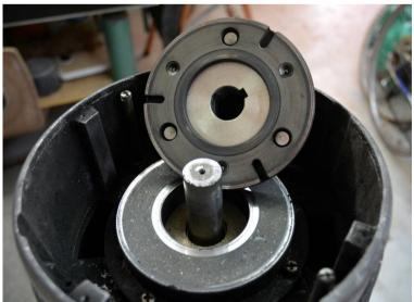
The brake on the end of the motor shaft prevented the fitting of a normal shaft mounted cooling fan so a separately powered fan was factory fitted, which is ideal for a VFD controlled motor because a motor powered fan does nor shift much air at low RPM.
