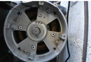
The missing brake gave me plenty of space in which to fit my brush idea. In my brushes and brush holders scrap box I found a suitable brass brush holder but no brushes that were meant for it, but I did have some with the right cross section but a short cable. The easy solution to this was to cut the brush holder to make it shorter. I used a piece of printed circuit board for mounting the brush holder because it was easy to solder the brass brush holder to it.
