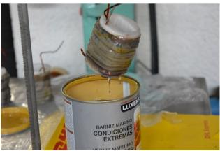
The coils were then left several days to thoroughly dry. In an attempt at reducing the core whine I smothered each leg with silicon sealer before fitting the coils back on and the "I" piece of the core was located externally with the sealer also. It does seem to be quieter but that is purely a perception from listening to it by someone predisposed to want that result.
