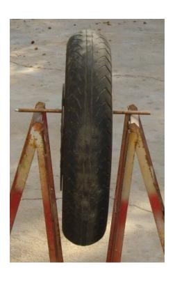
The previous photos show how the wheel needs to be mounted off centre such that it can swing from side to side about an axis defined by the supporting bar. In cases where there is no convenient symmetrical supporting locations (rear wheels and single disc fronts), the wheel can be supported by the bar just under the rim section.
