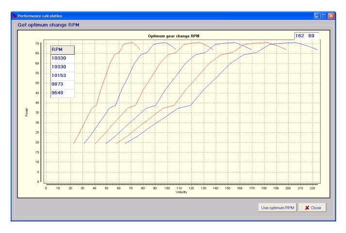
The "Get optimum Gears" button opens a window which allows for huge numbers of gear and sprocket ratio permutations to be calculated in only a few seconds.
