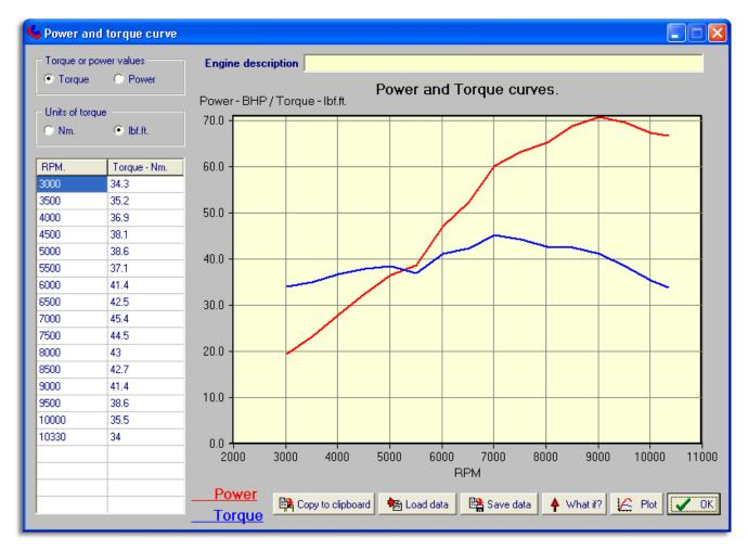
The data can be entered as either power or torques values against RPM. If "power" is selected then there is a units choice between BHP and kW, likewise if "torque" is the preferred input there is a choice of units between Nm and lbf.ft. All the internal calculations use Nm for torque but the conversion is taken care of inside the software. If you enter power data then the torque data will be calculated and vice versa.
