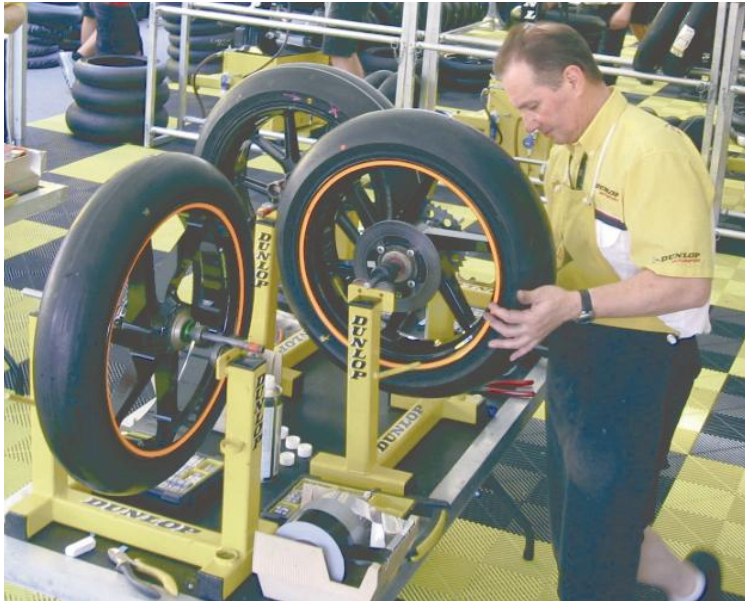
A typical scene at race meeting. A tyre technician is balancing a wheel statically. The relative narrowness of such wheels does not often allow for significant dynamic imbalance. Although the rear tyres of large racing machines are now of a width where it is becoming more likely that dynamic imbalance might cause problems.
