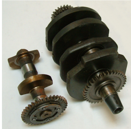
This typical balance shaft is fitted to a Kawasaki parallel twin cylinder engine with 180° crankshaft. Such a crankshaft already has perfect primary balance but creates a rocking couple due to the separation of the two cylinders. In this case the balance shaft is there to smooth out that couple.
