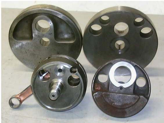
Fig. 3 Different methods of reducing the metal mass on the crankpin side of the crankshaft. The top left hand example is typical of forged wheels. It is common with wheels machined from the solid to drill holes.
