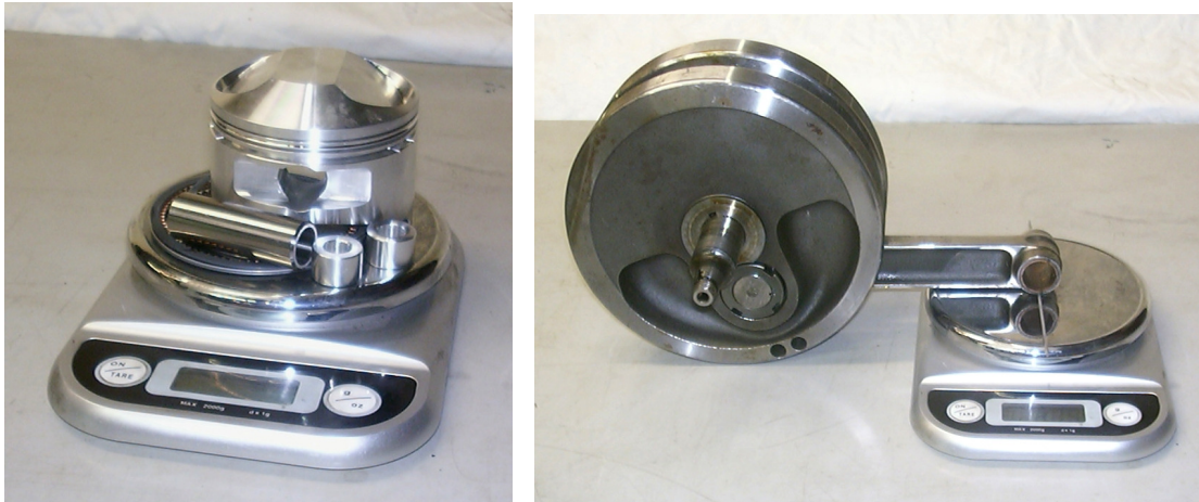
Fig. 5 Weighing the reciprocating masses. Although the piston, etc. could be mounted on the conrod for these measurements to get the total reciprocating mass, we would still need to separate out the weight of the conrod little end in order to calculate the mass to be added for balancing.
